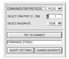
If the baudrate should be changed, a connection must first be established by clicking on **TRY TO CONNECT**.
