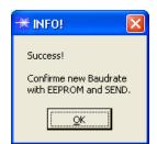
When the new baudrate information has been successfully sent, the sensor operates with the new baudrate. A window will pop up, prompting you to select **EEPROM** and then to press **SEND**. After a hardware reset the new baudrate only will be used when **EEPROM** and **SEND** have been pressed.
