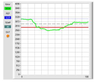
When the current measurement value **RAW** (green line) rises above the hysteresis threshold (black line) again, the output **OUT0** changes to +24V again (signal is OK). This is visualised by the **OUT** LED.
