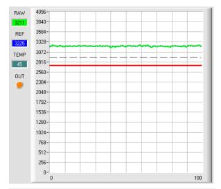
As long as the current measurement value **RAW** (green line) lies above the switching threshold (red line), the output **OUT0** is at +24V (signal is OK). This is visualised by the **OUT** LED.
