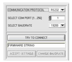
The baudrate for data transfer through the RS232 interface can be set by means of the **SELECT BAUDRATE** drop down menu and **CHANGE BAUDRATE** function field.
