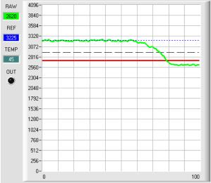
When the current measurement value **RAW** (green line) falls below the switching threshold (red line), the output **OUT0** changes to 0V (error). This is visualised by the **OUT** LED.
